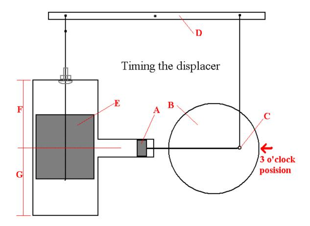
With the "Power Piston" (A) all the way out of the power cylinder, The connecting point (C) on the "Flywheel" (B) should be all the way to the right or the 3 o'clock posision. The "Walking Beam" (D) should be level. The "Displacer Piston" or "Displacer" (E) should be in the middle of it's travel up and down. In other words dimention **F** should be the same as dimention **G**.
